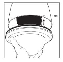
Remove the two lower dome, mounting screws. Apply a drop of Loctite (supplied) to each screw.  d. Push the lower dome inside the back box, line up the mounting screw holes, and install the two mounting screws.
